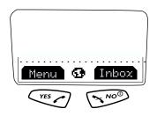
To use the soft key functions, press the left (YES) or right (NO) key that is under the text label on the screen. The soft keys on your phone's screen override the key names. For example, press YES to select Menu or press NO to select the Inbox.
